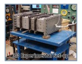
**HOCAM** also conducts <u>ADVANCE</u> thermal recovery experiments with <u>3D experimental set-ups</u>; to mimic multi-phase fluid flow, heat and mass transfer behavior better at reservoir conditions, to optimize well location and orientation; horizontal and vertical well orientations.
